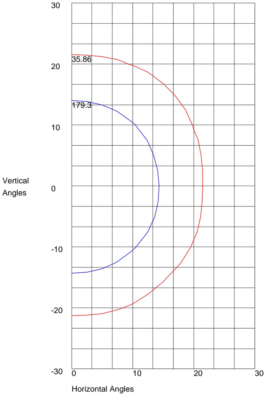
Maximum Candela = 358.6 Located At Horizontal Angle = 0, Vertical Angle = -5
