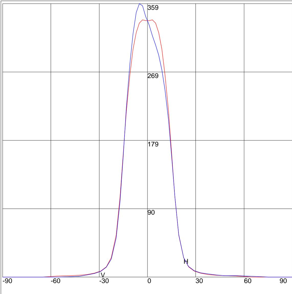
Maximum Candela = 358.6 Located At Horizontal Angle = 0, Vertical Angle = -5
