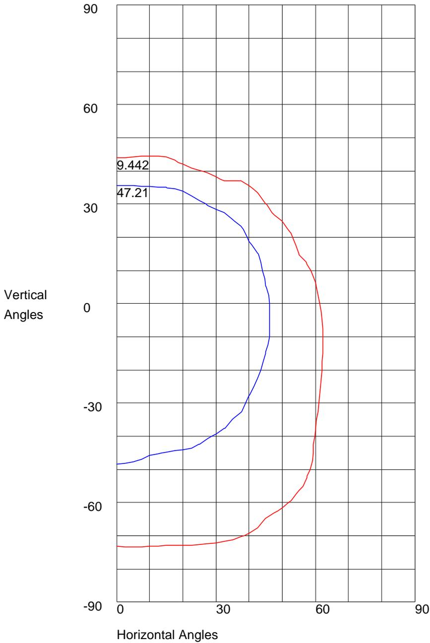
Maximum Candela = 94.42 Located At Horizontal Angle =-3, Vertical Angle =-3
