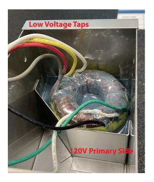
**Step 5:** Reassemble power supply, test operation. Finished.
