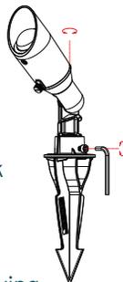
main wire lead running to the transformer, keeping most of the excess wire at the fixture. Bury excess wire directly at the base of the fixture.
