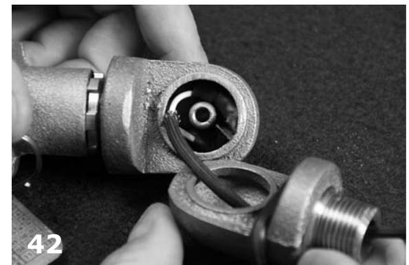
42 Retract socket wire to allow reassembly.
