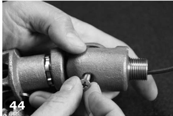
44 Re-insert screw and tighten.
