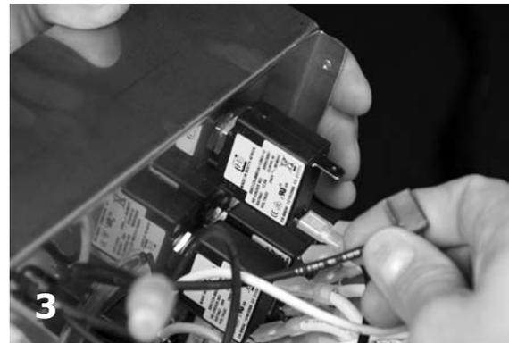
Locate breaker on back side and remove wires.
