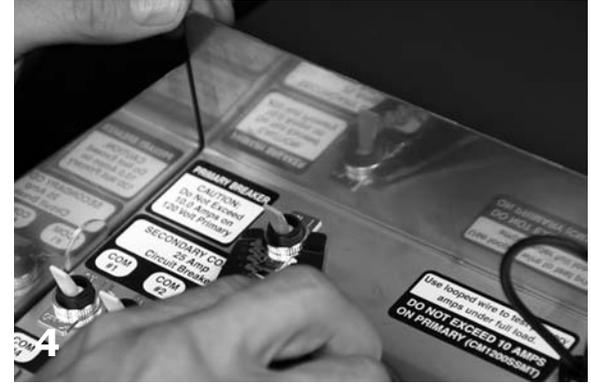
On panel face, loosen breaker set screw.
