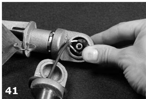
41 Press crimps into wire channel.
