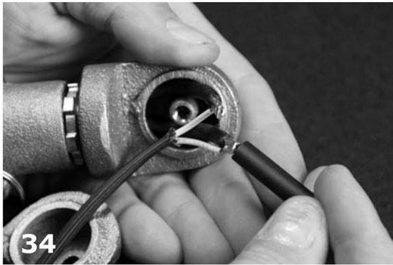
34 Slip heat shrink tube over crimp and wire.
