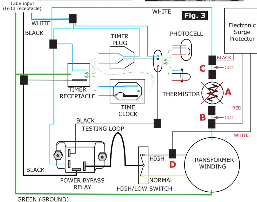
**CAUTION:** Unplug the transformer from the 120V outlet before opening the internal transformer compartment. 120V conductors are exposed during this replacement procedure. Utilize an electrician if statutes, regulations or codes require you to do so.
