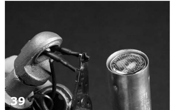
39 Using pliers, compress heat shrink past crimp.
