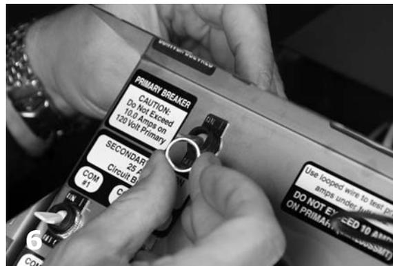
Insert new beaker. Replace plate and set screw.
