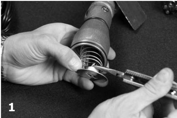
1 Remove shroud and heat reflector.
