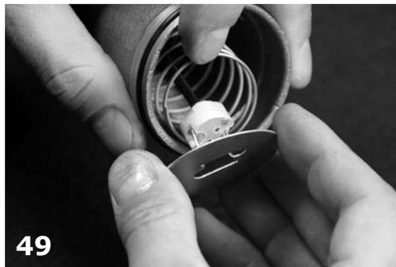
49 Insert heat reflector into socket head.
