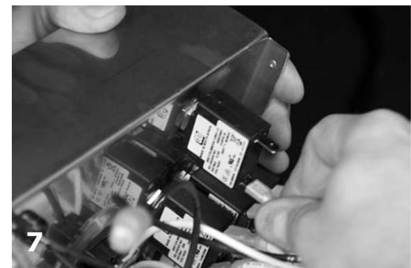
Reattach wires. Lower and secure inner panel.
