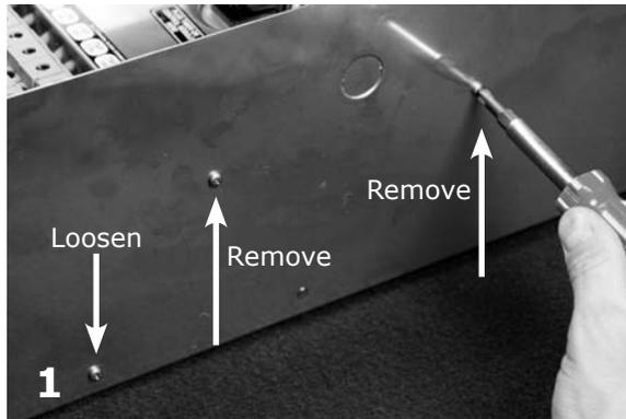
1. Remove and loosen screws from each side.
