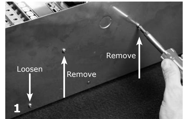
Remove and loosen screws from each side.
