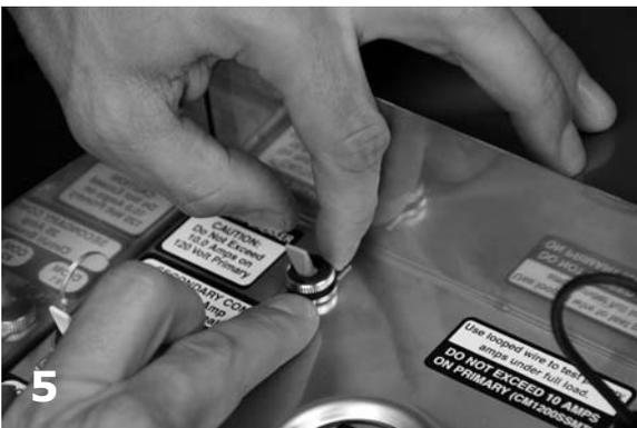
Remove set screw and plate. Remove breaker.
