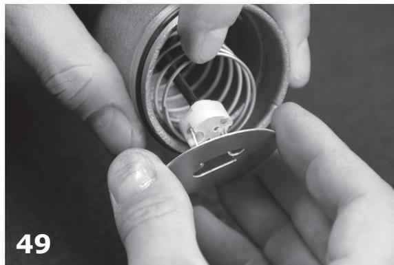
49 Insert heat reflector into socket head.
