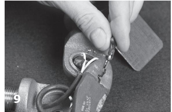
9 Cut wire junction on wire-side of crimp.
