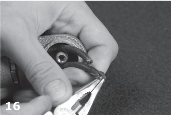
Using pliers, remove old heat shrink.
