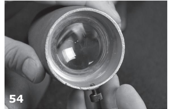
Before applying shroud, retract set screw so it does not extend past inside shroud surface.
