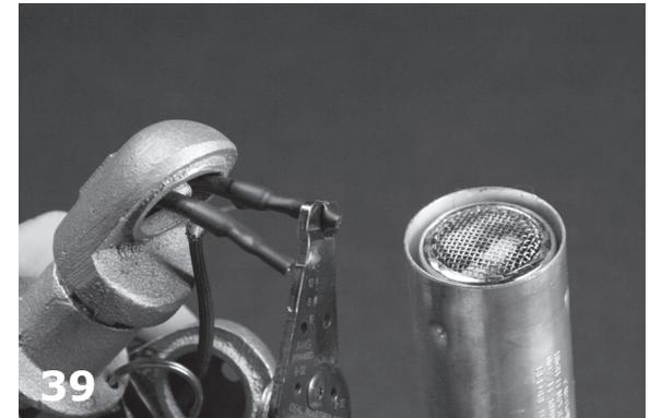
Using plier, compress heat shrink past crimp.
