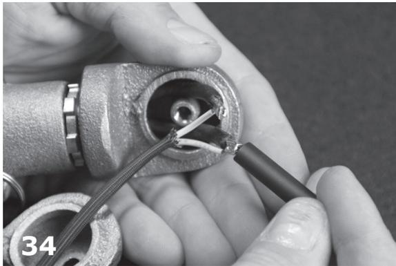
Slip heat shrink tube over crimp and wire.
